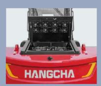
The integrated fan cooling system ensures the stability of the electric control system, and the fully opened hood
